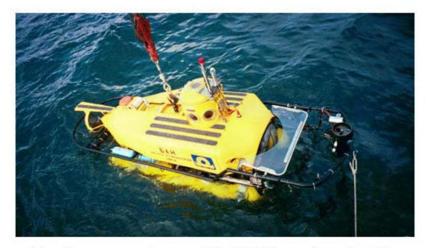
The 3-person submersible *PC-8B*, equipped with a scanning sonar, lights, an underwater video camera, and manipulator, is capable of diving to depths of 250 meters.
